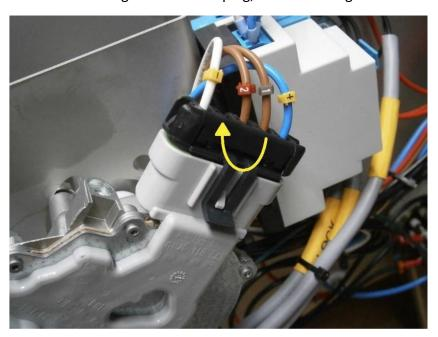
The brown wire, located at the second terminal from the right, must be moved to second terminal from the left (which is now unused).
