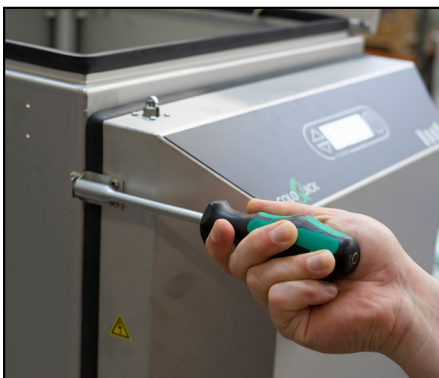
16. Close the lid and mount the nuts to lock the service door.
