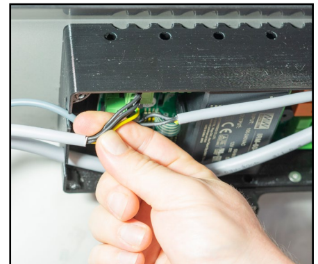
9. Locate the green connector on the top of the board. BE CAREFUL TO CHOOSE THE CORRECT CONNECTOR!
