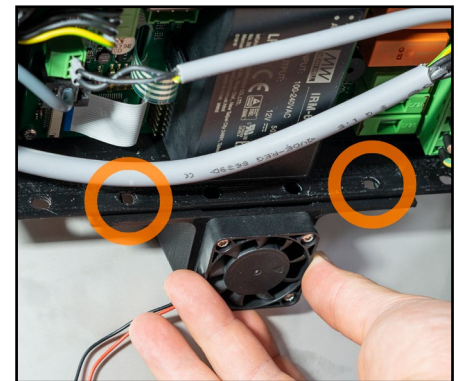
6. Align the screw holes of the fan unit with the holes in the black box. Make sure to push the fan unit as far back as possible.
