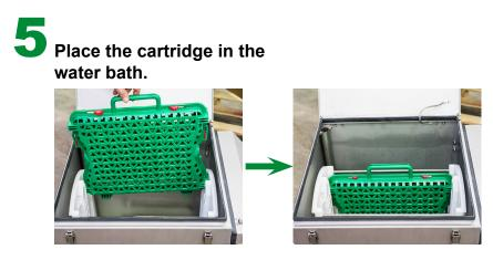
\*The machine is shown without water in the water bath for information purpose only. Always make sure there is water in the wather bath before turning the thawing unit on. Press to remove the cartridge from the water bath.
